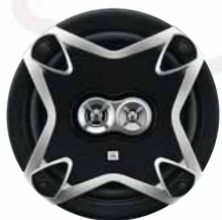
GT5-803 200mm (8") 3-Way Coaxial System • Power handling, RMS: 70W • Power handling, peak: 210W • Frequency response: 40Hz – 20kHz • Sensitivity: 92dB • Impedance: 4 ohms • Mounting depth: 77mm (3-1/16")
